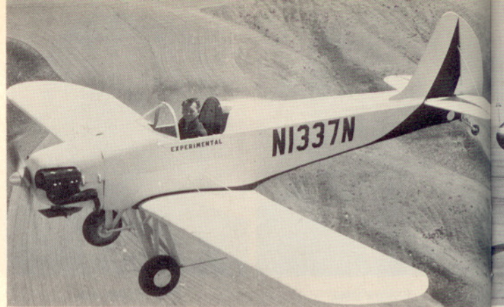
FIGURE 2 Use of registration on fuselage became optional during Korean War. Note separate lettering by cockpit to indicate experimental status following deletion of second letter from registration. (Airplane is the Story homebuilt, powered by a 65 h.p. Continental engine.)
