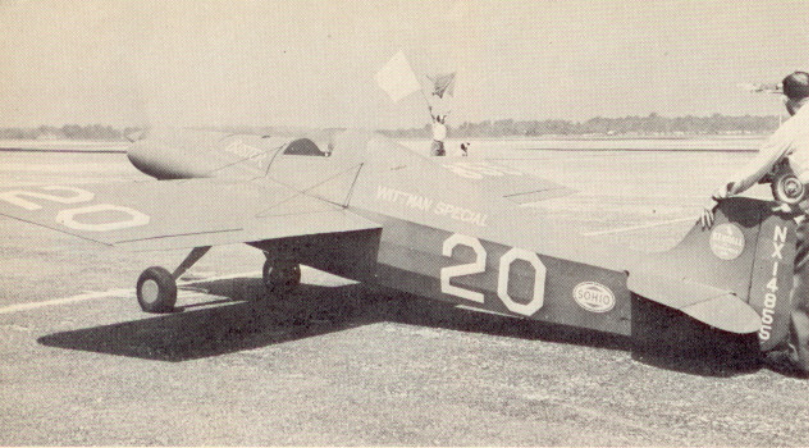
FIGURE 1 Standard position of racing numbers. Second number of registration was deleted in 1949 but could be retained on fabric-covered planes until next repainting or covering. (Airplane is Steve Wittman's original "Buster" of early 1930's, rebuilt as 85 h.p. Goodyear racer in 1947, which is now in the National Air Museum.)
